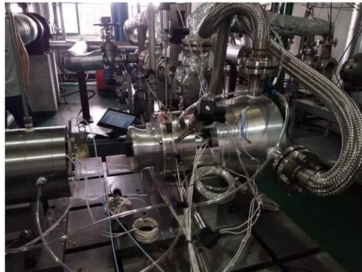
**Figure 8: Photo of Stand-Alone Spin Test Rig Platform for E100F GTE**
