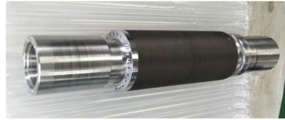
**Figure 1: Alpha Hardware Connected to Induction Motor through Flexible Coupling (Left); Alpha Generator Shaft Assembly (Right)**
