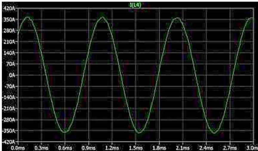
**Figure 2: Ripple Current on Simulated Motor Current Waveform with Three-Level MLI & Sine Filter**
