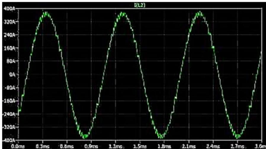
**Figure1: Ripple Current on Simulated Motor Current Waveform With Two-Level Inverter**
