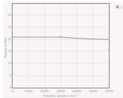
Power vs. Speed & Torque vs. Speed Charts for an e+a Constant Torque, PM Generator
