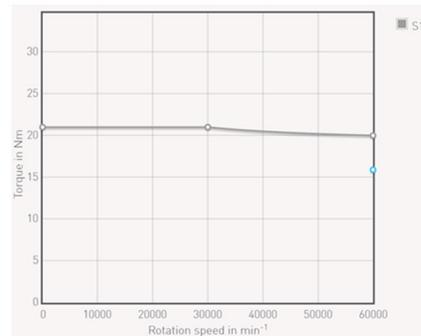
Power vs. Speed & Torque vs. Speed Charts for an e+a Constant Torque, PM Generator
