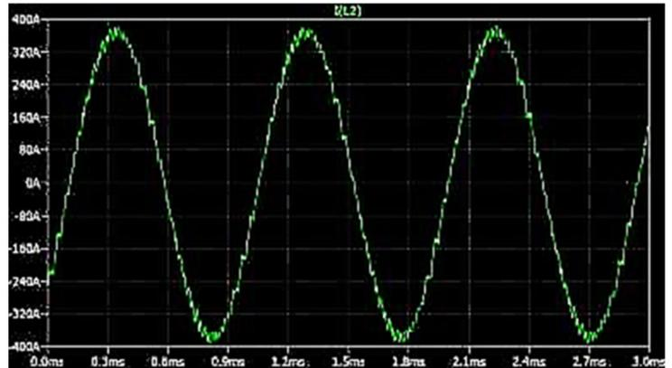
Simulated Ripple Current in a 2-Level Inverter:
