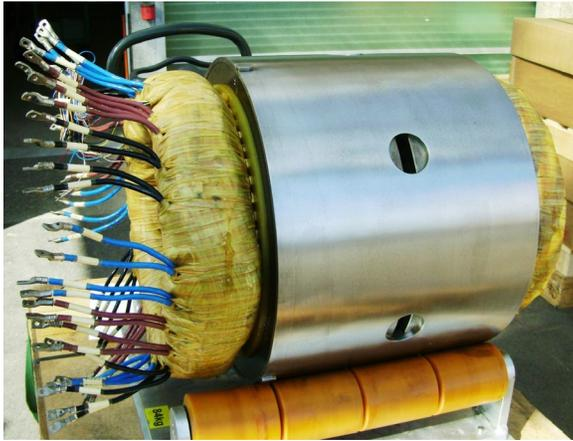
1.6MW, 25K RPM Stator for
