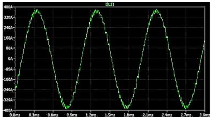
Simulated Ripple Current in a 2-Level Inverter:
