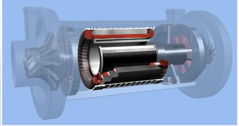
Conceptual Drawing of e+a Rotor & Stator w/Cooling Jacket
